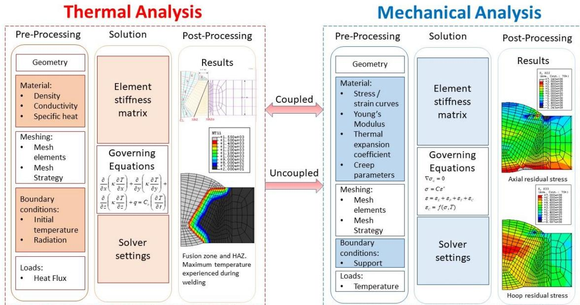
Figure 6: General scheme for RS calculation using FEM.
