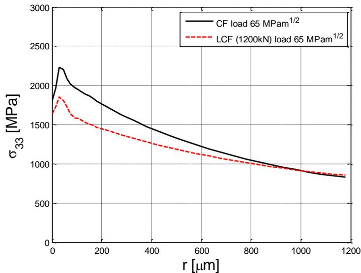
Figure 11: Opening stress in front of the macroscopic crack tip for a CF load cycle and a LCF load cycle.
