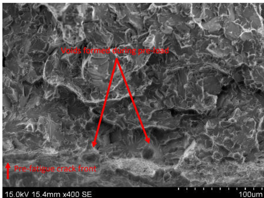
Figure 12: SEM picture with magnification of 400 times, fracture specimen subjected to a LUCF load transient [43].
