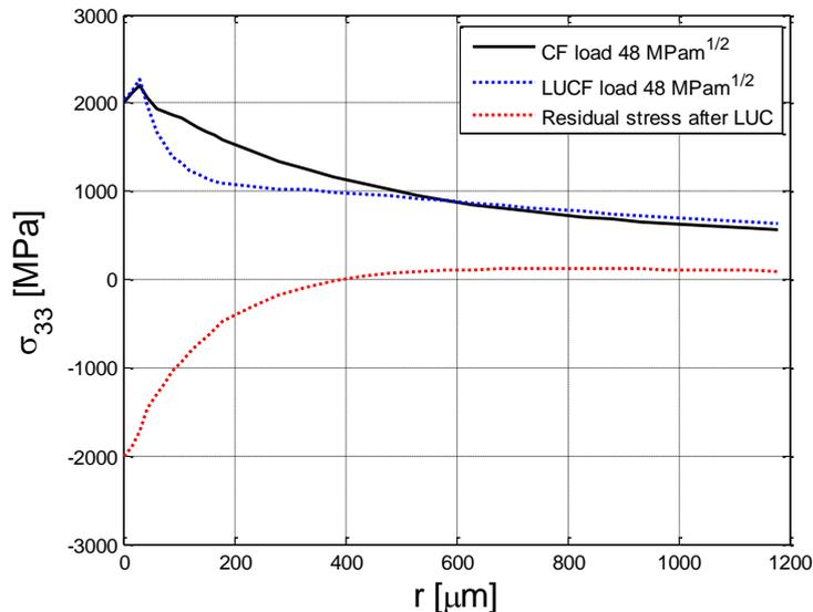
**Figure 10: Opening stress in front of the macroscopic crack tip for a Cool-Fracture (CF) cycle and a Load-Unload-Cool-Fracture (LUCF) load cycle after cooling and reloading.**
