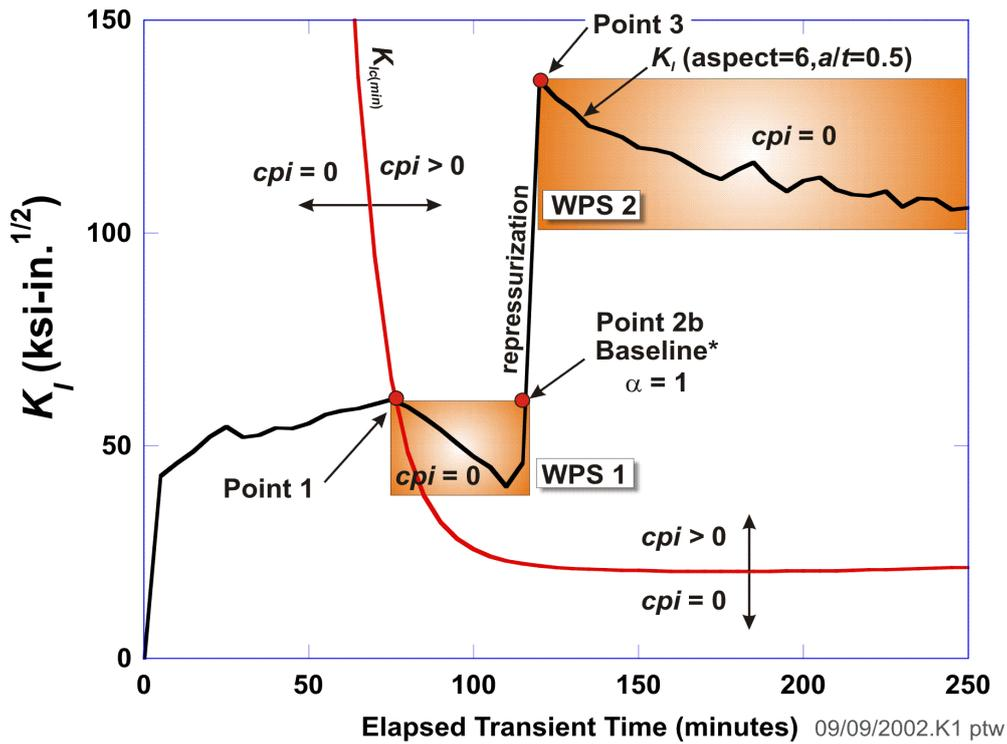
Figure 18: Example of warm prestressing: load path for a flaw showing two WPS regions. (*cpi* is the instantaneous conditional probability of initiation).
