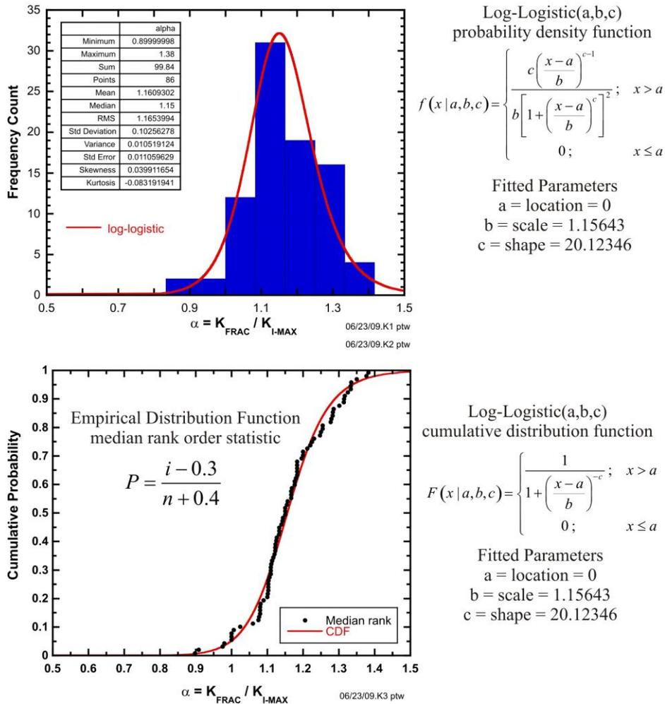
Figure 16: Example of warm prestressing: log-logistic distribution fitted to data obtained from Moinereau et al. [16] for a parameter in Best-Estimate Model for warm-prestress model implemented in FAVOR.
