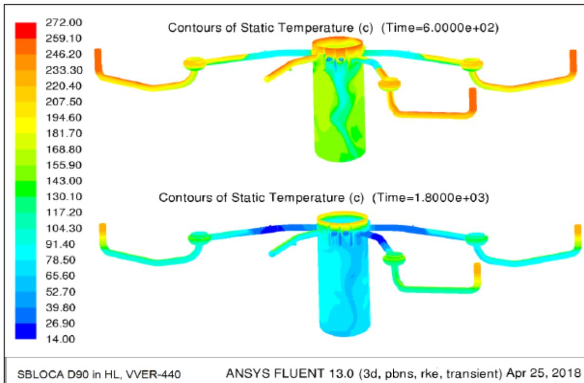
Figure 41: CFD mixing analysis of SBLOCA in VVER-440 [107].
