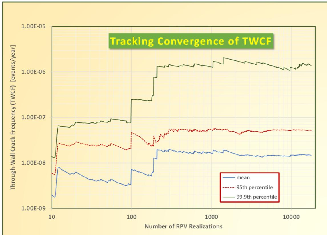
Figure 33: Tracking convergence of TWCF as a function of RPV realizations.
