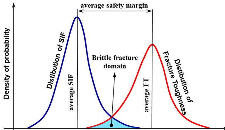
**Figure 37: Scheme for conditional probability determination.**
