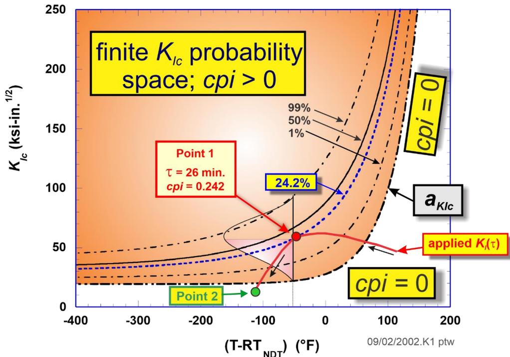
Figure 39: Interaction of the applied  $K_I$  time history and the Weibull  $K_{Ic}$  statistical model.
