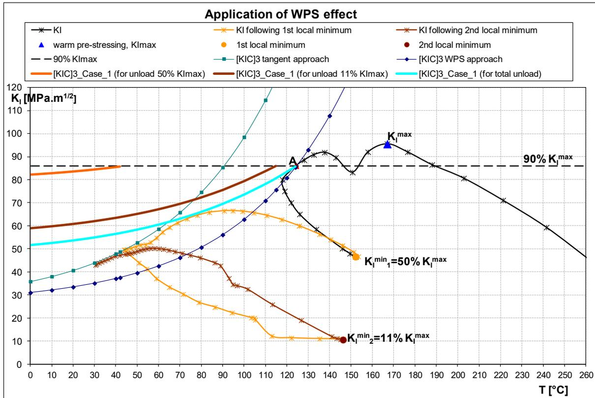
Figure 13: Illustration of the procedure for WPS approach application according to NTD AME.
