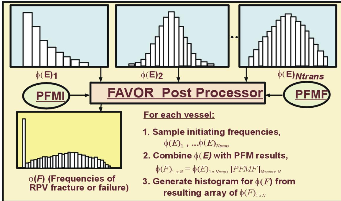
**Figure 31:** The FAVPost module combines the distributions of conditional probabilities of initiation and failure calculated by FAVPFM with initiating frequency distributions for all of the transients under study to create distributions of frequencies of RPV initiation of fracture and RPV failure.
