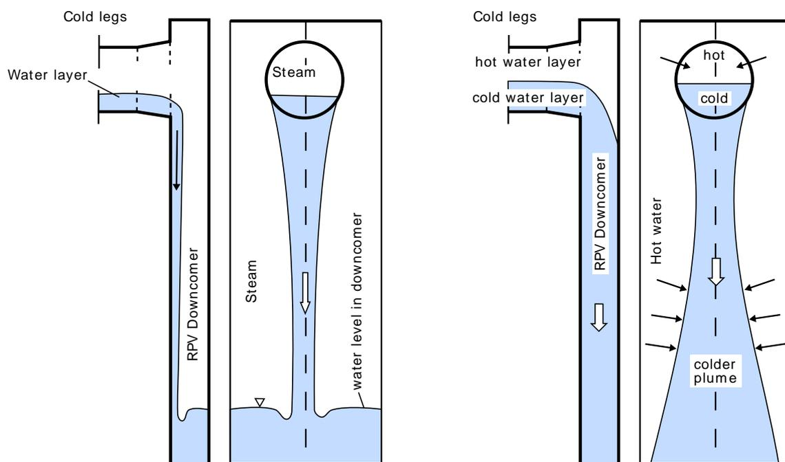
Figure 23: Stripe cooling (left part) and plume cooling (right part) of the RPV inside wall [6].
