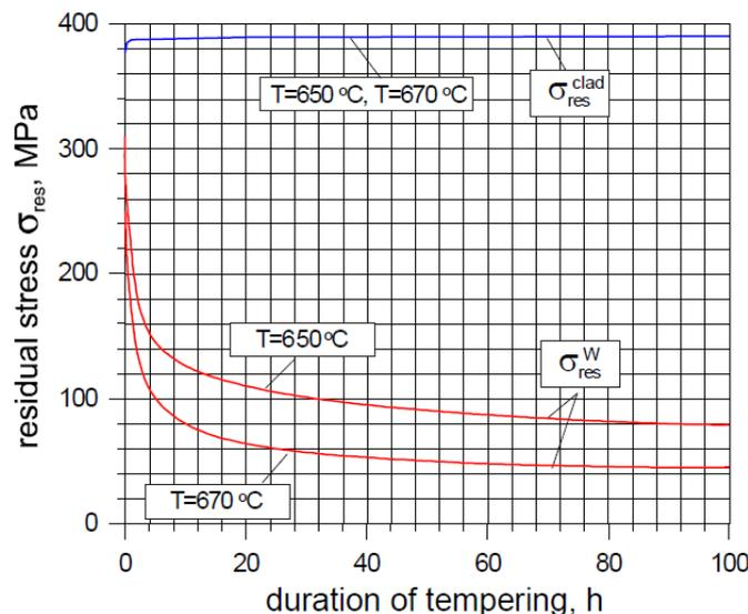
**Figure 3: Dependency of RS magnitude on duration and temperature of tempering.**
