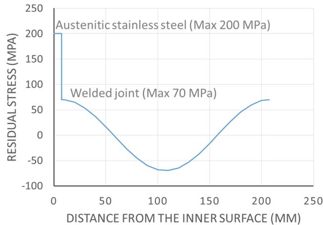
Figure 5: RS profiles as a function of distance from the inner surface.
