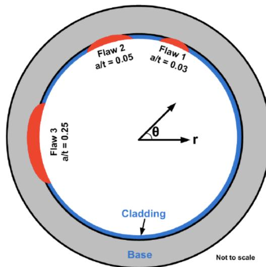
Figure 8: Schematic of three inner-surface breaking flaws of interest with varying depth and constant aspect ratio of flaw length to depth (figure not to scale).
