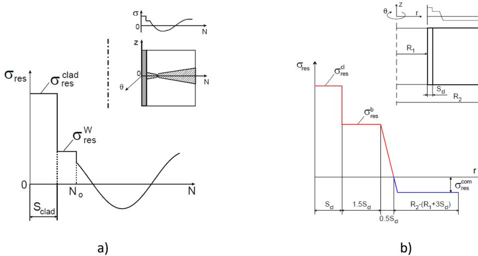
**Figure 2: RS profile through the RPV wall thickness in a) weld, b) base metal.**
