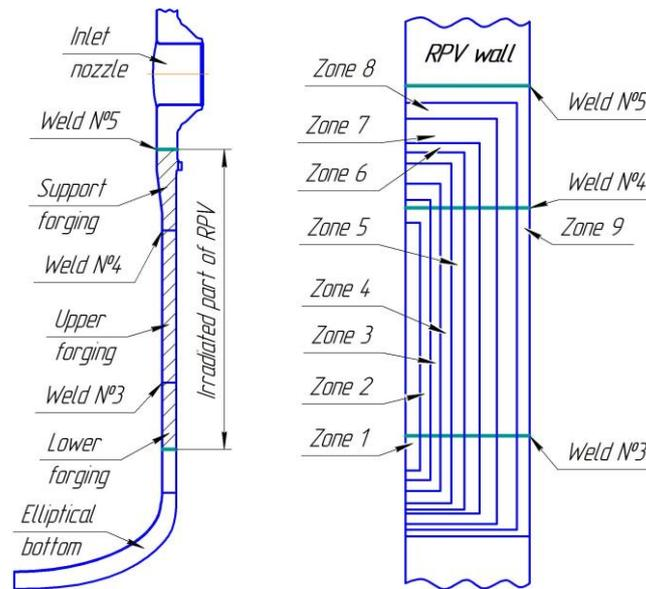
**Figure 38: WWER-1000 RPV (without outlet nozzle and flange) and layout of its radiated part on estimated zones.**
