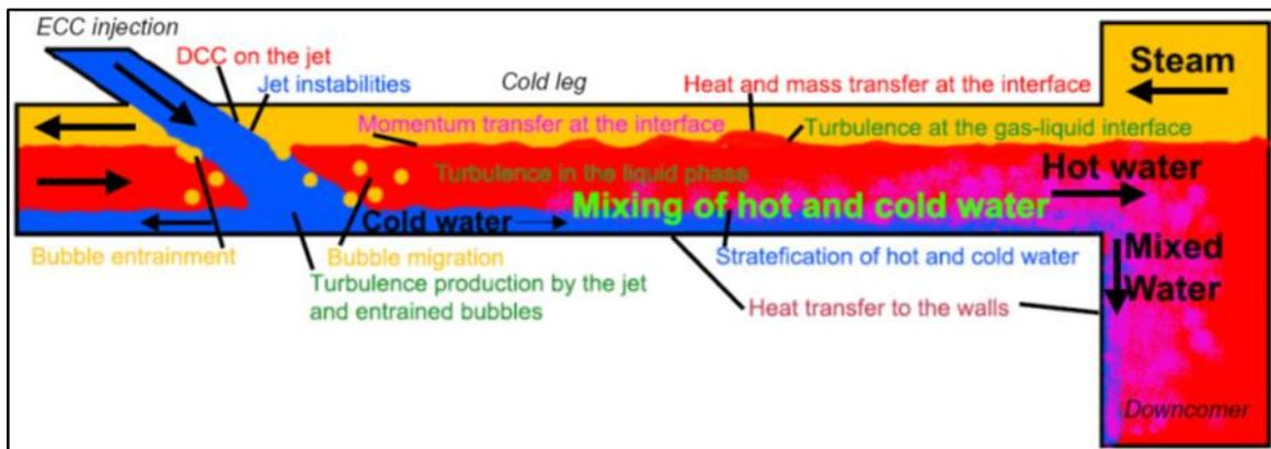
**Figure 24: Thermal stratification in cold leg and forming of cold plume in downcomer[36].**
