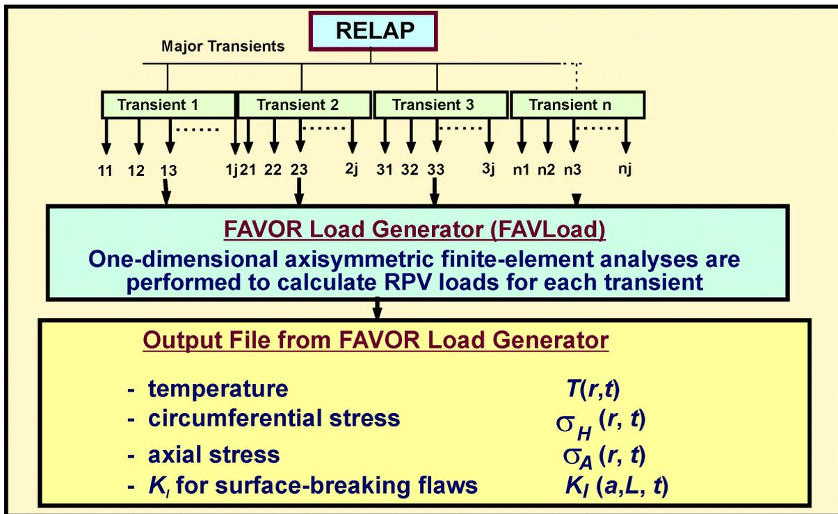
Figure 28: The FAVOR Load Generator performs deterministic analyses for a range of thermal-hydraulic transients.
