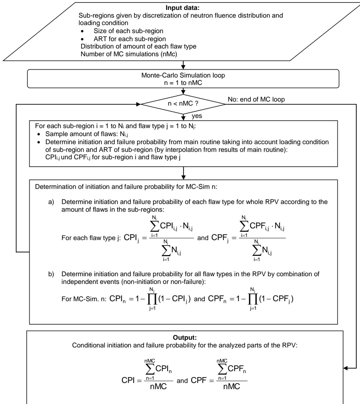
Figure 26: FRA-G in-house tool – Post-Procedure.
