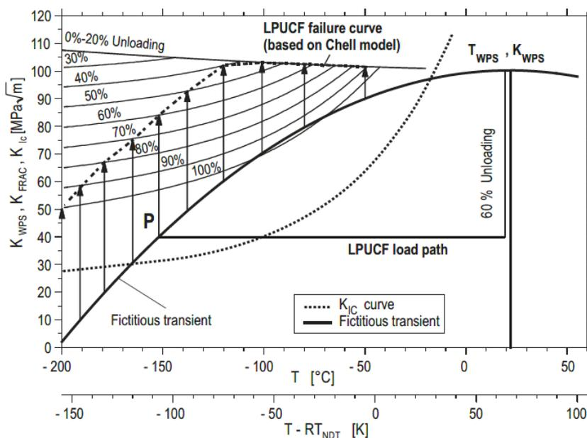
Figure 14: Principle sketch to show the determination of the fracture toughness  $K_{FRAC}$  upon warm pre-stressing.
