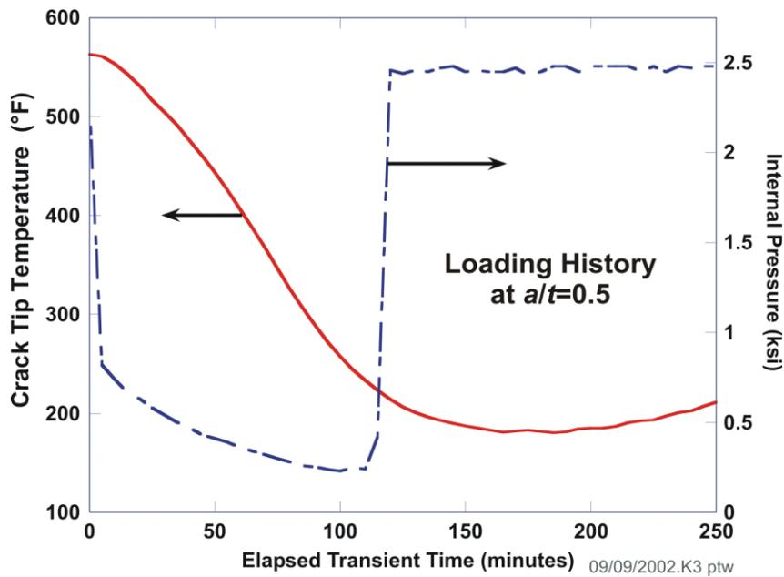
Figure 17: Example of warm prestressing: loading history with pressure applied to the inner surface and the temperature at the crack tip.
