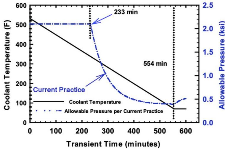
Figure 7: Prescribed pressure-temperature limits for normal cool-down transients determined using standard ASME code procedures. Results are shown for Vessel A at 60 EFY with a cool-down rate of 27.8 °C (50 °F/hr).
