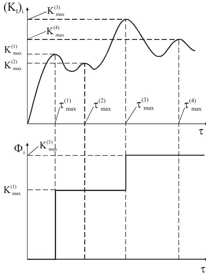
**Figure 21: Scheme illustrating the  $\Phi_i(\tau)$  function determination based on a known  $(K_I)_i$  dependence on time  $\tau$  [25].**
