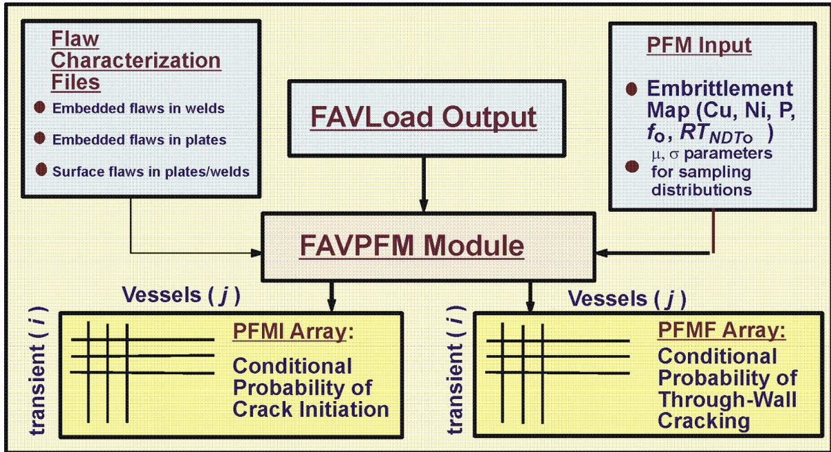
Figure 29: The FAVPFM module takes output from FAVLoad and user-supplied data on flaw distributions and embrittlement of the RPV beltline and generates PFMI and PFMF arrays.
