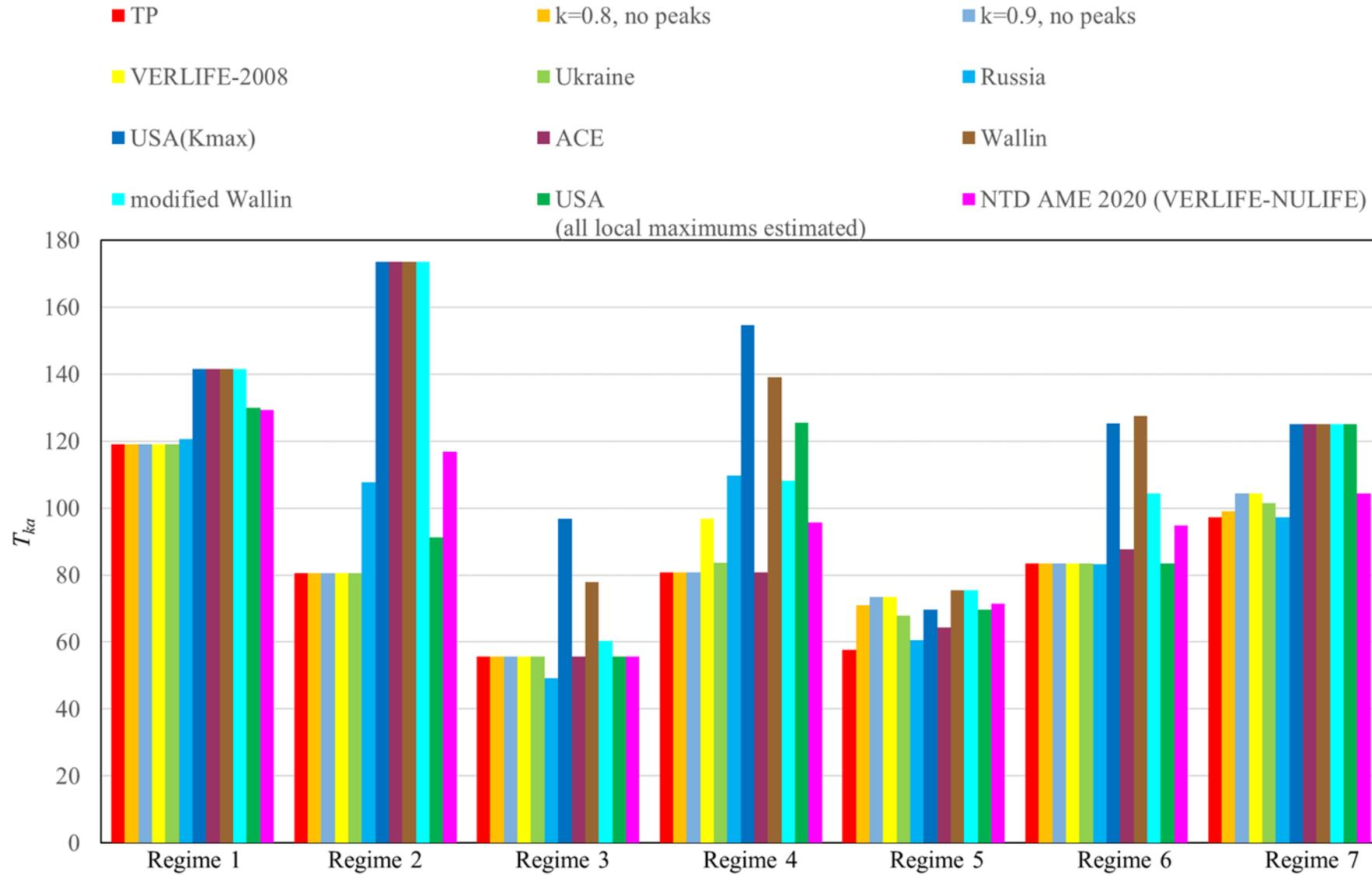
Figure 22: Variation of the maximum allowable transition temperature for considered transients depending on the WPS model applied.
