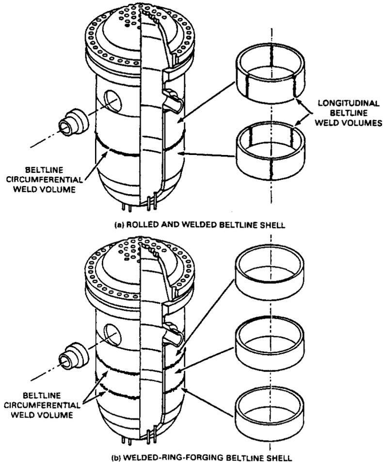
Figure 1: Fabrication configurations of PWR beltline: (a) rolled-plate construction with longitudinal and circumferential welds and (b) ring-forging construction with circumferential welds only.
