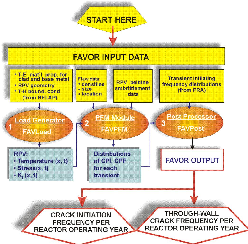
Figure 27: FAVOR data streams flow through three modules: (1) FAVLoad, (2) FAVPFM, and (3) FAVPost.
