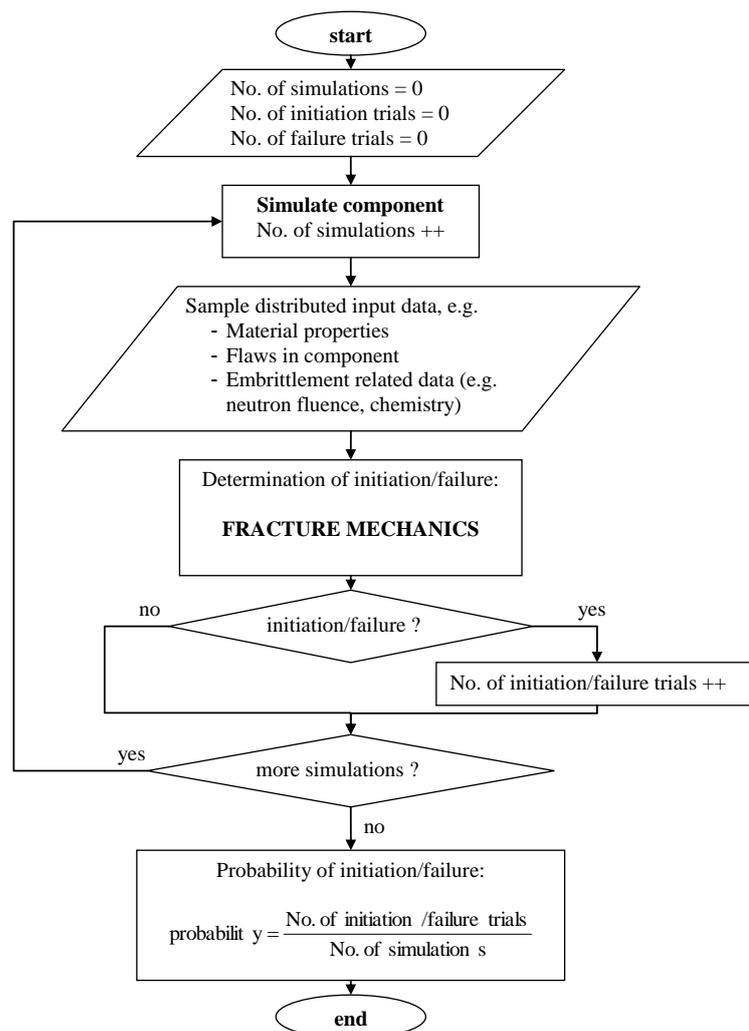
**Figure 40: Flow chart of standard Monte Carlo method for fracture mechanics assessment.**
