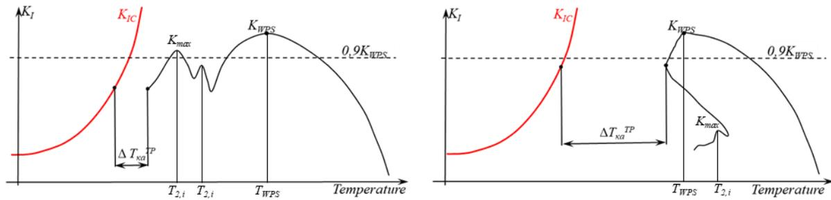
Figure 15: PTS examples for which WPS is not applicable according to the Ukrainian rules [12] (TP denotes tangent point method).
