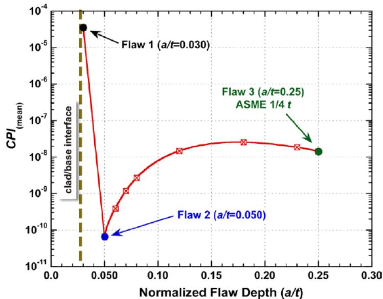
Figure 9:  $CPI$  for circumferentially oriented, inner-surface flaws exhibiting non-monotonic behavior with flaw depth for Vessel A subject to the pressure and temperature limits determined from the standard ASME code procedure and shown in Figure 7, the latter is based on 60 EFPY and cool-down rate of 50 °F/hr [110].
