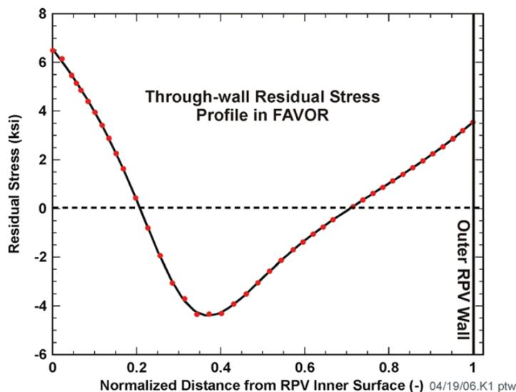
Figure 4: Welding residual stresses in FAVOR 16.1 [13].
